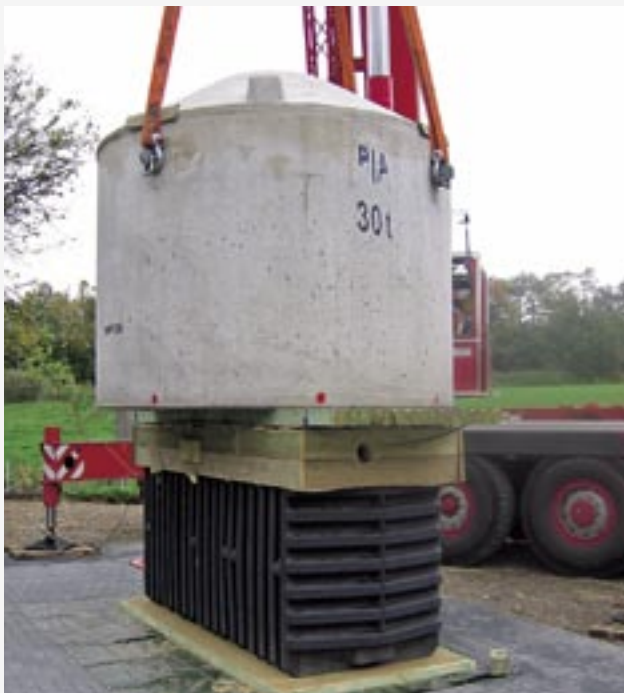
For your safety: Extreme load tests are an important component of the quality assurance.
